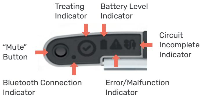
The Battery Level, Error/Malfunction and Circuit Incomplete indicators also have an accompanying vibration and audible buzzer in case the icons are not visible.
