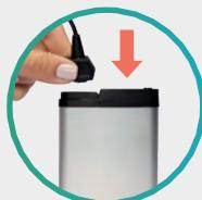
Connect the other end of the generator lead wire (largest block) to the generator.
